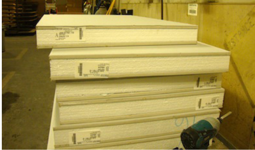
Before Test: Sandwich Panels
